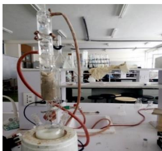
Figure-2 Extraction of the seed oil using Soxhlet apparatus
